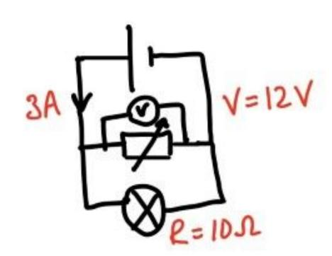
Calculate the resistance of the variable resistor.
