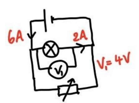
Calculate the resistance of the variable resistor.
