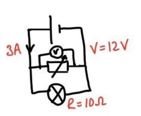
Calculate the resistance of the variable resistor.
