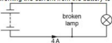
Noah says that when the broken lamp is replaced the 4A current will be shared between the two lamps, so each gets 2A. The total current from the battery will still be 4A. (You may assume that the lamps are alike.)
