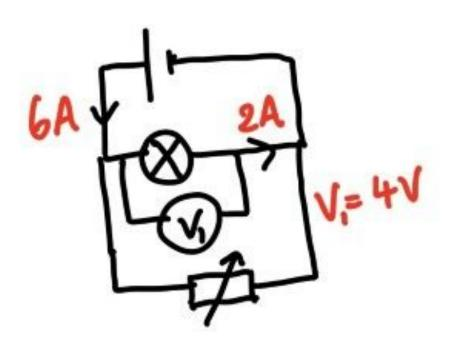
Calculate the resistance of the variable resistor.
