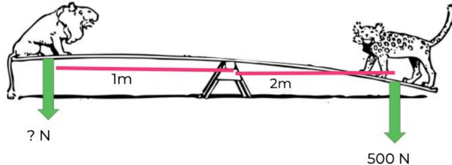
$$\begin{aligned} \text{Clockwise moment} &= \text{Anticlockwise moment} \\ \text{Force x distance} &= \text{Force x distance} \end{aligned}$$
