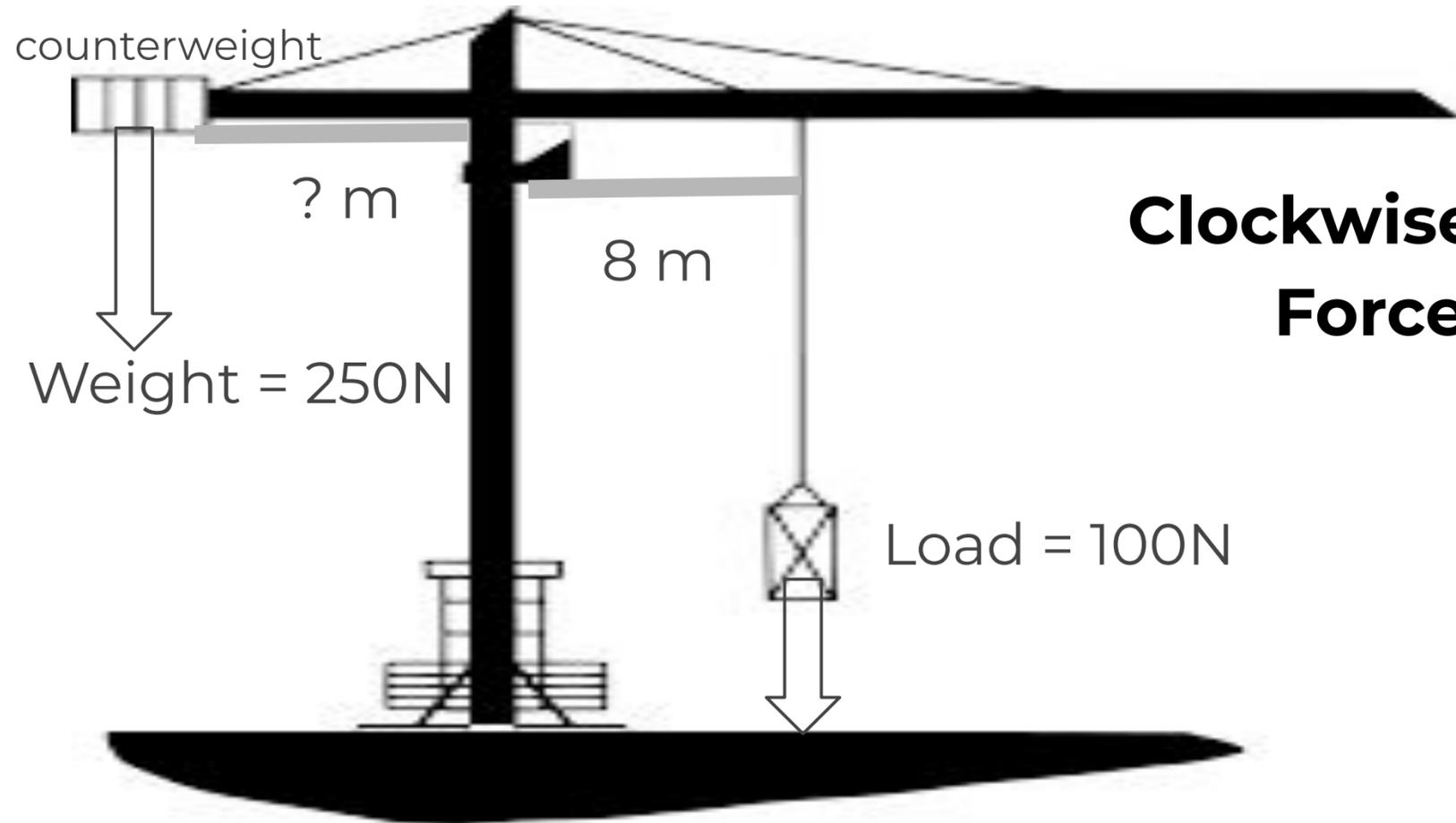
$$\begin{aligned} \text{Clockwise moment} &= \text{Anticlockwise moment} \\ \text{Force x distance} &= \text{Force x distance} \end{aligned}$$
